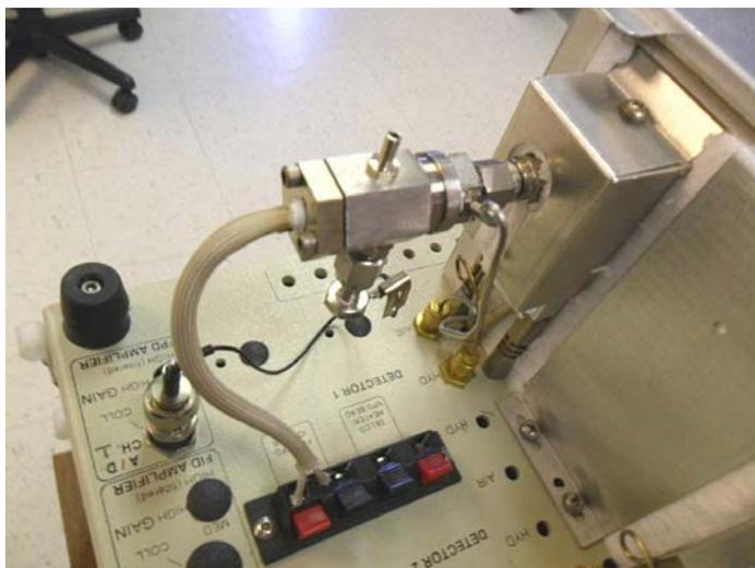
SRI Instruments GC – DET tower attaches to 1/8 inch diameter jet via a Swage fitting. 1/16 inch side Swage port adds Air flow to detector. Custom signal probe arm extends 1.5 inches from tower and bends down in unshielded bare wire.
