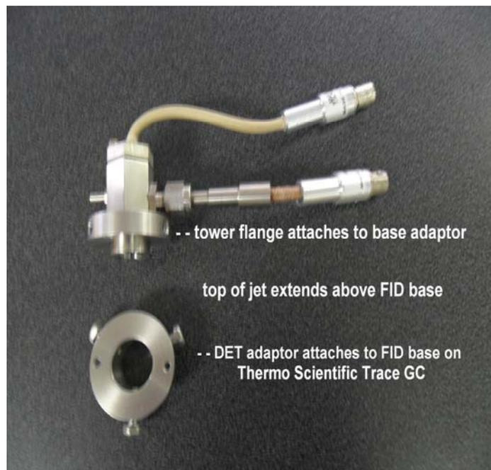
Thermo Trace Ultra GC – custom fits Thermo base. Signal probe terminates in an SMA type connector.
