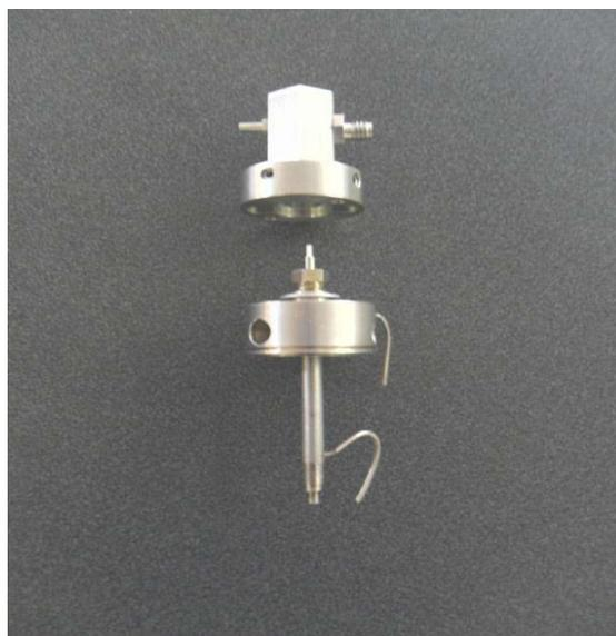
**Figure 23.** DET retrofit tower mounts onto Varian/Bruker base with 2 short screws, and includes a ceramic tipped jet that seals with a stainless steel ferrule.
