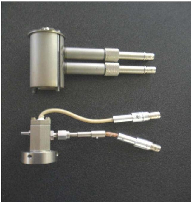
**Figure 22.** Varian/Bruker NPD at top, DET retrofit NPD/TID/CCID/FID equipment at the bottom.
