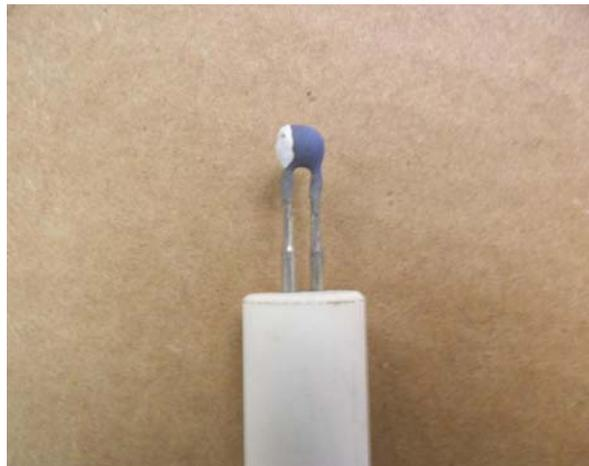
**Figure 21.** DET hybrid coating for Varian/Bruker NPD bead.
