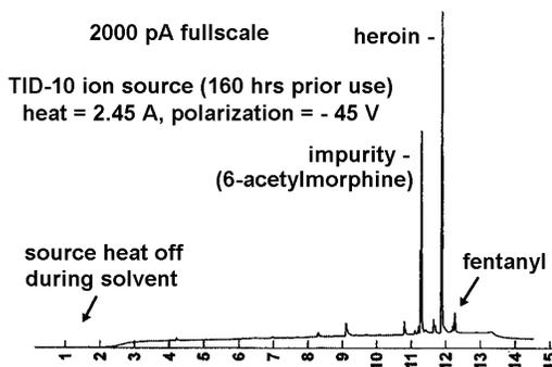
**Figure 2.** Same sample as Fig. 1. Detector gases for TID-10: N2 through "Air" line=60, N2 makeup=10 mL/min, N2 through "H2" line= setting of 2.
