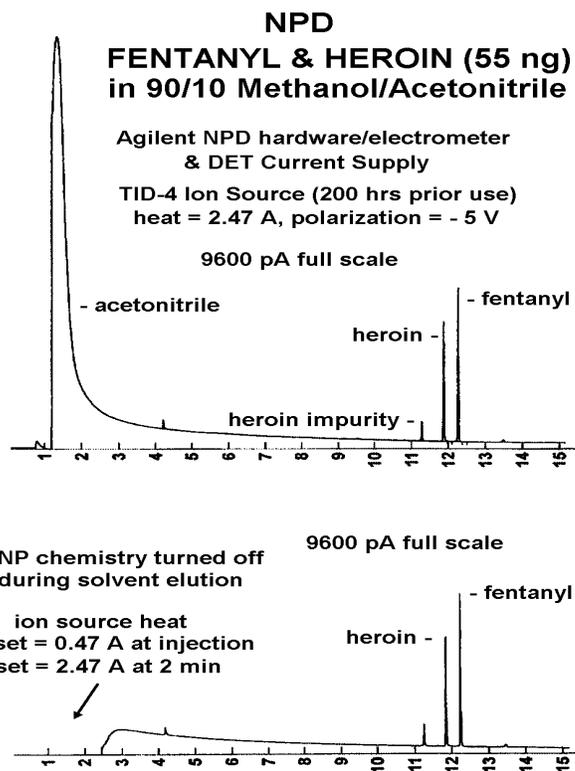
**Figure 1.** column: 30m x 0.32mm x 0.25µm DB-5ms, He=4mL/min, 100 - 300degC at 15degC/min. detector gases: H2=3, Air=60, N2 make up=10mL/min
