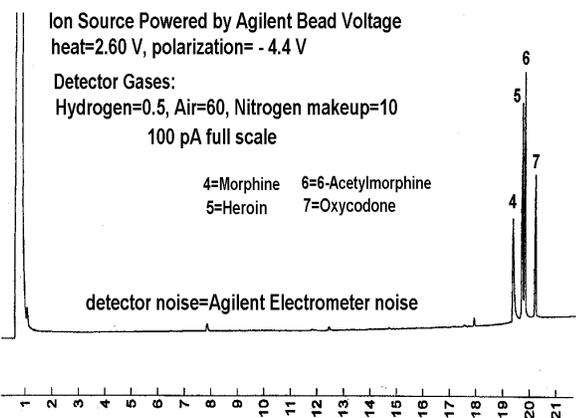
**Figure 7.** Same column as Figure 6. 110-300°C at 10°C/min, 300°C - 2 min.
