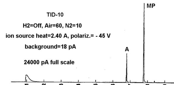
Figure 10. TID-2, TID-3, TID-5, and TID-10 are DET ceramic ion sources with different catalytic ionizing surface formulations for different compound selectivities. Same column as Fig.1, He=3, 100-250°C at 15°C/min.
