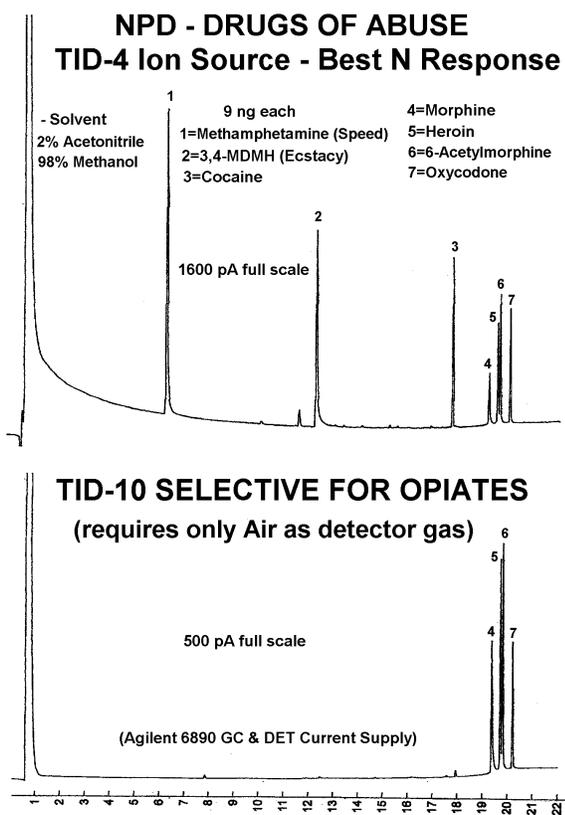
Figure 4. 30m x 0.53mm x 1.5µm DB-5ms, He=10mL/min 90-170°C at 7°C/min, 170-310°C at 16°C/min, 310°C-2min
